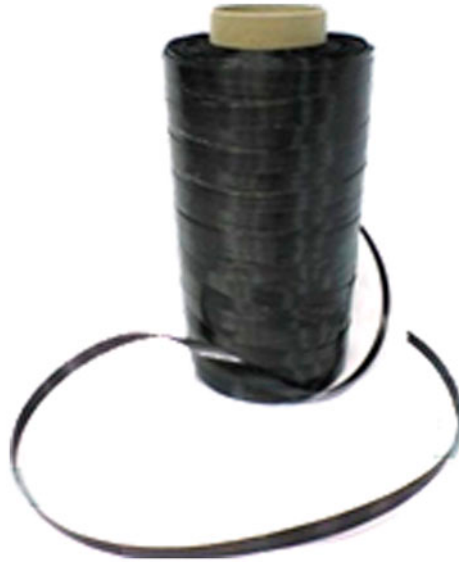
Figure 1. Prepreg tape of carbon fiber and polypropylene.
